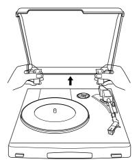
**2** Remove the lid, and set the voltage selector to the local power line voltage using a screwdriver.
